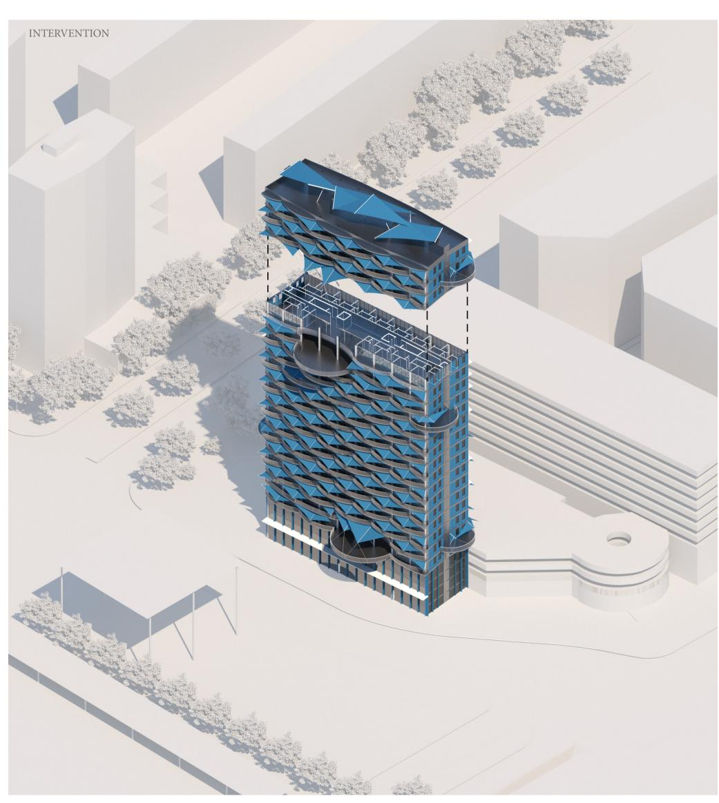
The proposal aims to decompact the existing building by creating open outdoor spaces at different heights with varying degrees of pri-vacy through terraced structures embedded in the framework and a pergola system that will help support them and provide solar protec-
